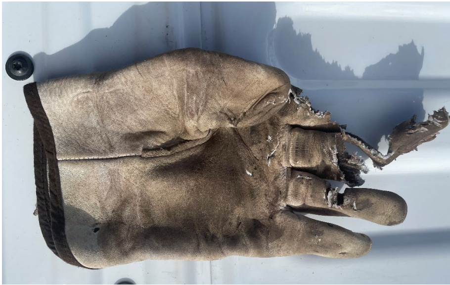
Figure 2: Sawyer's left glove showing damage from chainsaw.
